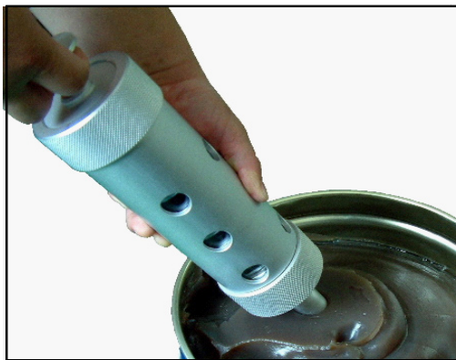
a. Insert an injection port into the Grease
