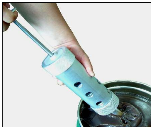
b. Pull the handle and wait for 2seconds (Grease gets into the inside of pump)
