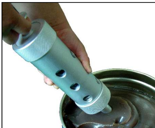
a. Insert an injection port into the Grease
