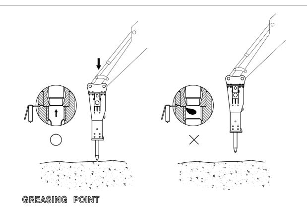
The greasing point on the hammer have been marked with the following sticker.
