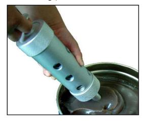
a. Insert an injection port into the Grease
