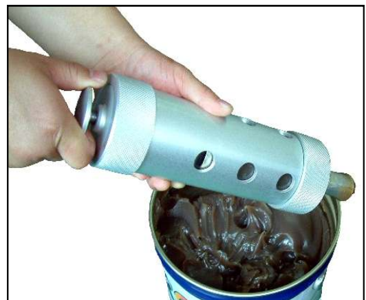
e. When grease is sufficiently filled fasten the handle by turning it clockwise
