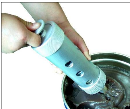
c. Inset the handle (Grease becomes compressed in the refilling cartiedge)
