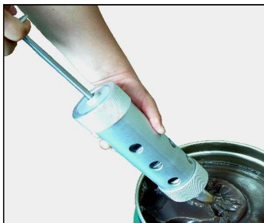
b. Pull the handle and wait for 2seconds (Grease gets into the inside of pump)
