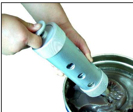
c. Inset the handle (Grease becomes compressed in the refilling cartridge)
