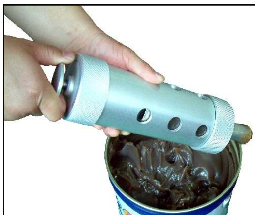
e. When grease is sufficiently filled fasten the handle by turning it clockwise
